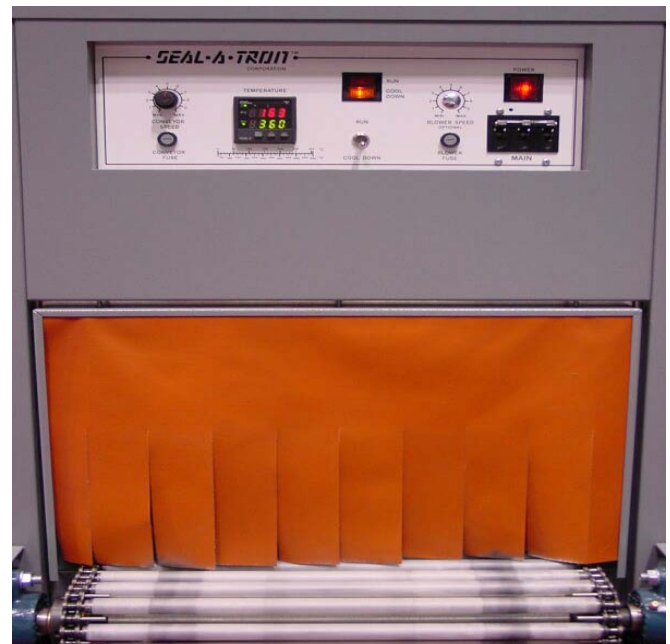
The Control Panel is located above the infeed of the Shrink Tunnel to be operated from both sides.
