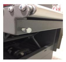
Use a 7/16 wrench to turn the adjustment bolt 1/8 turn at a time. Tightening the left adjustment bolt will make the conveyor belt move to the right. And tightening the right adjustment bolt will move conveyor to the left. It is advisable to try and get the conveyor belt running closer to the seal bed and away from the timing belt.
